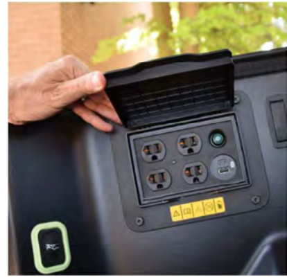
Figure 25 - Ford F-150 Lightning Power Outlets Accessible from Front Trunk (Autoweek)
